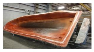
Manufacturing begins with the forming of two fiberglass hulls – an outside hull and an inner hull. A rigid layer of Foam is placed between the two hulls and they are permanently fastened together with a confidential material and process. This results in a hull that is over an inch thick and very strong. The seats, cabin, roof, and other fittings are all assembled to the hull, usually with screw or bolt fasteners. In several places a heavy sheet of aluminum is embedded
