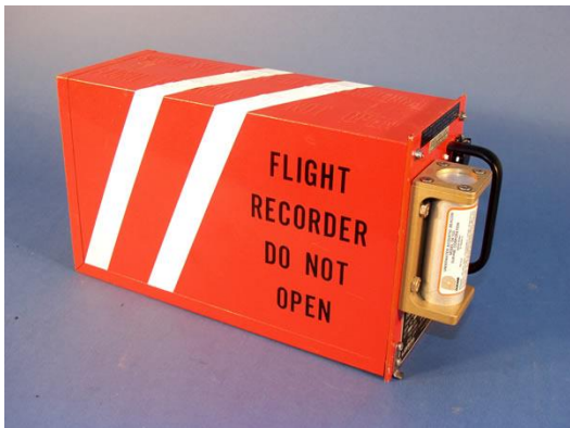
One of the two “black boxes” in an Aircraft: the all-important flight data recorder
