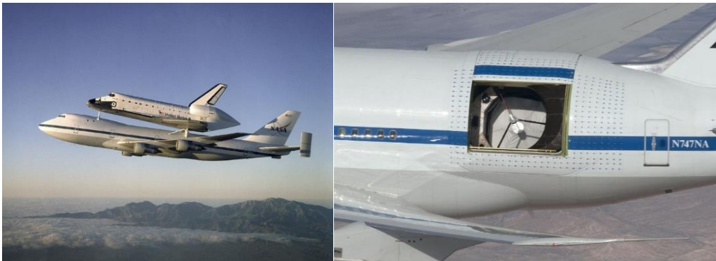
The Shuttle Carrier Aircraft, SCA An airborne telescope on a 747 by NASA
