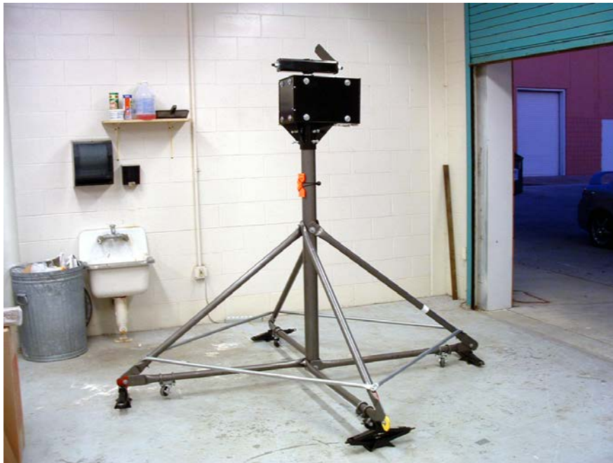
Figure 2 - SRT Pedestal with AZ/EL Gearbox Attached in the Development Lab at ERAU
