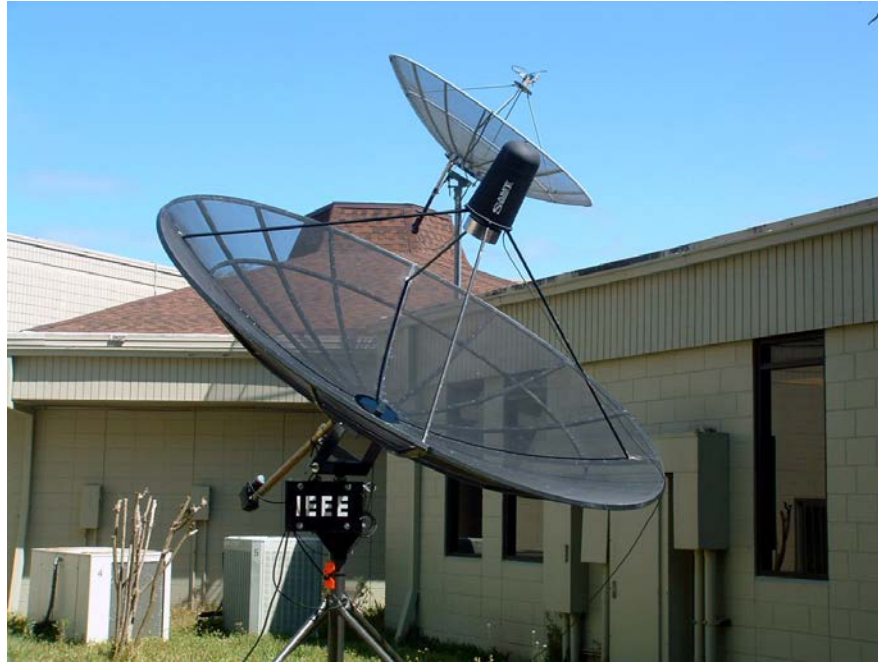
Figure 22 - The SRT shown during Initial Sun Tracking Tests with the newly installed 10 foot Parabolic Reflector
