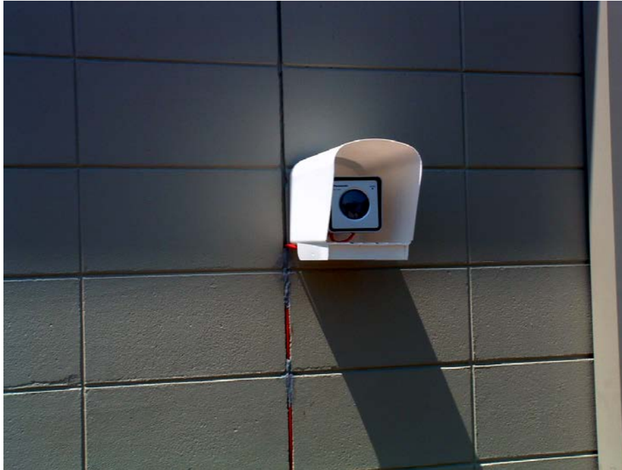
Figure 44 - Webcam Mounted on the Exterior to Monitor Physical Position of the SRT Antenna Structure
