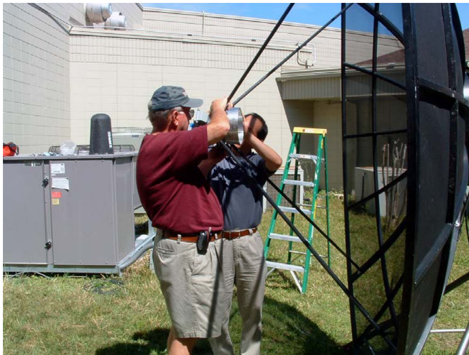
Figure 21 - Al Jusko and Dr. Liu adjusting the focal distance from the subreflector to the main reflector in the new configuration
