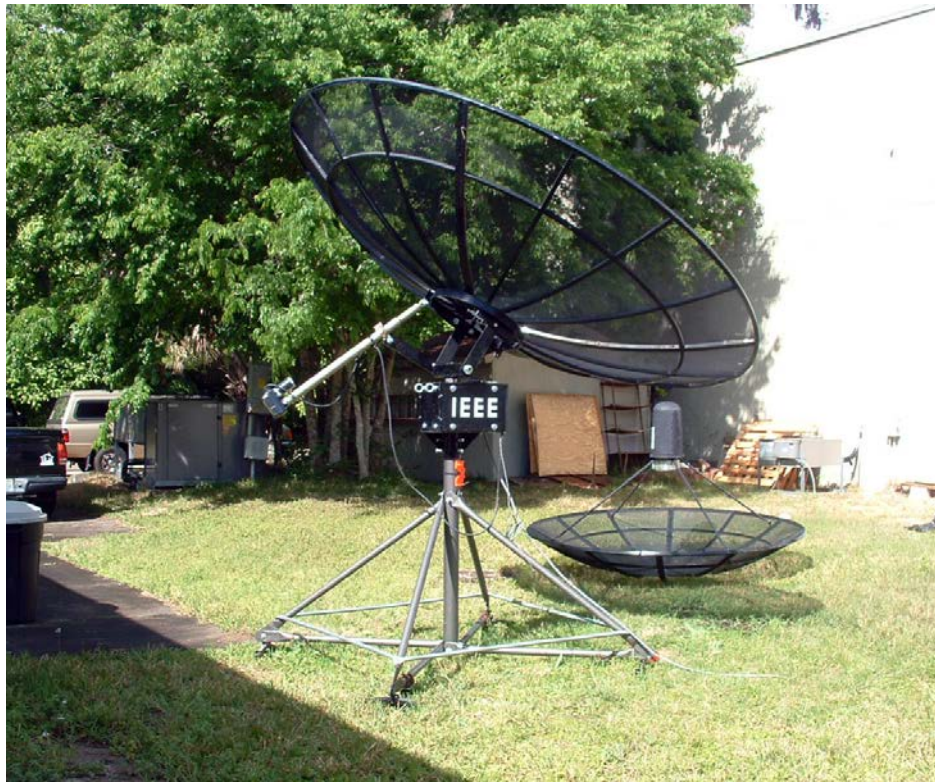
Figure 20 - The SRT with the new 10 foot parabolic dish bolted into the halo ring.
