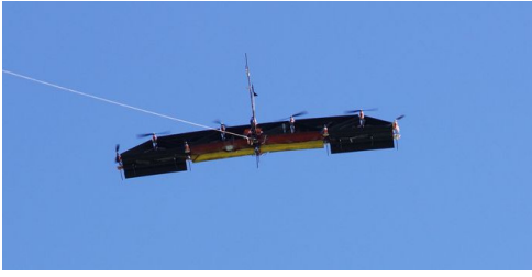
Fig. 2. Demonstrator of an Airborne Wind Turbine (AWT) system of Joby Energy [9].
