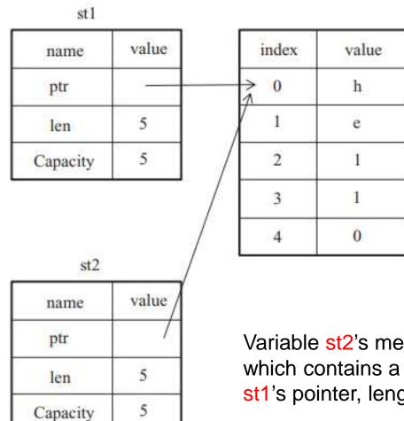
Variable st2's memory representation, which contains a duplicate of st1's pointer, length, and capacity.
